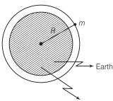
Orbital speed of the satellite orbitting the earth is given by  $v_o = \sqrt{\frac{GM}{R}}$
