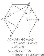
Force on mass m at A due to mass m at B is,  $f_1 = \frac{Gmm}{r^2}$  along AB.
