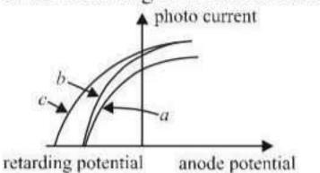
(a) Curves (a) and (b) represent incident radiations of same frequency but of different intensities.
