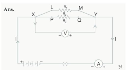
It is observed that the total current I, is equal to the sum of the separate currents through each branch of the combination.
