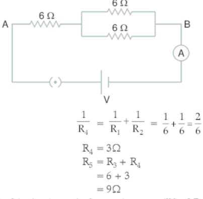
In this circuit, equivalent resistance will be  $9\Omega$ . (ii)  $4\Omega$
