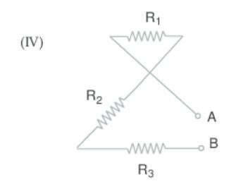
Ans. Figure I and IV have series combinations only. Resistance are placed between terminal A and B only.
