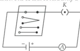
Now, plug the key. Note the current in the ammeter. Now replace the wire by a thicker nichrome wire, of the same length. A thicker wire has a larger cross-sectional area. Again note down the current through the circuit. Instead of taking a nichrome wire, connect a copper wire in the circuit. Again note down the current.
