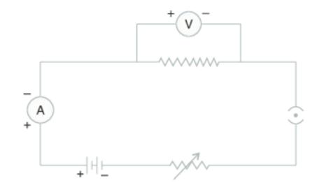
A device to regulate current without changing the voltage source in an electric circuit is called a variable resistor or a rheostat.
