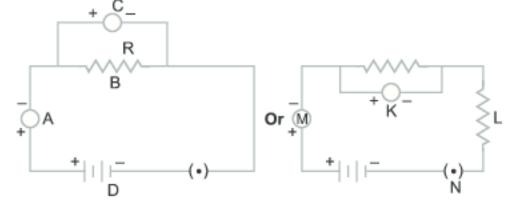
Ans. M or A = Ammeter, L or B = Resistance, K or C = Voltmeter, D = Potential difference, N = Key  $\frac{1}{2} + \frac{1}{2} + \frac{1}{2} + \frac{1}{2}$
