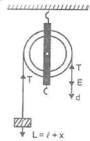
Single fixed pulley system consists of a single pulley. It is attached to some high platform and around its groove passes a rope. One end of rope is attached to the load and the effort is applied at the other end.
