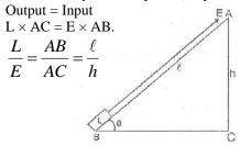
$$\therefore MA = \frac{Length \ of \ inclined \ plane}{Height \ of \ plane} = \frac{\ell}{h}$$
