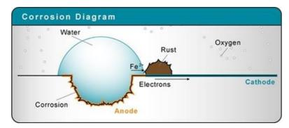
For example, reddish brown color rust is form on iron rod when it comes in water contact this is called as corrosion
