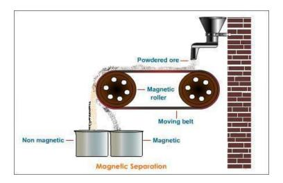
The powdered ore is dropped over a conveyor belt running over two rollers, one of which is magnetic. The magnetic ore particles get attracted to the magnetic roller and run along with the conveyor belt for a little longer than the non magnetic gangue. Gangue particles drop down first forming a heap. Then, the magnetic ore particles drop down forming a separate heap. Thus, two separate heaps of ore and gangue particles are formed.
