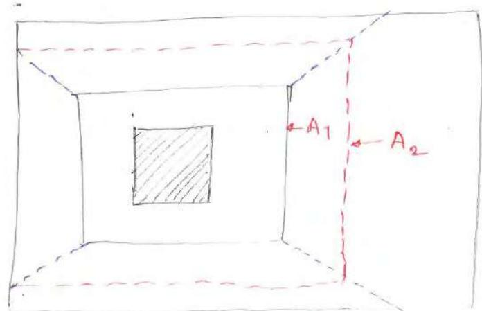
Bearing strength of concrete is enhanced by  $\sqrt{\frac{A_2}{A_1}}$
