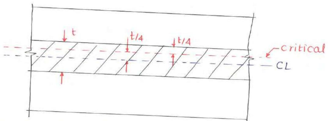
3. If footing slab is supporting a steel column with gusset plate then critical section is at the mid of face of column and edge of gusset plate.
