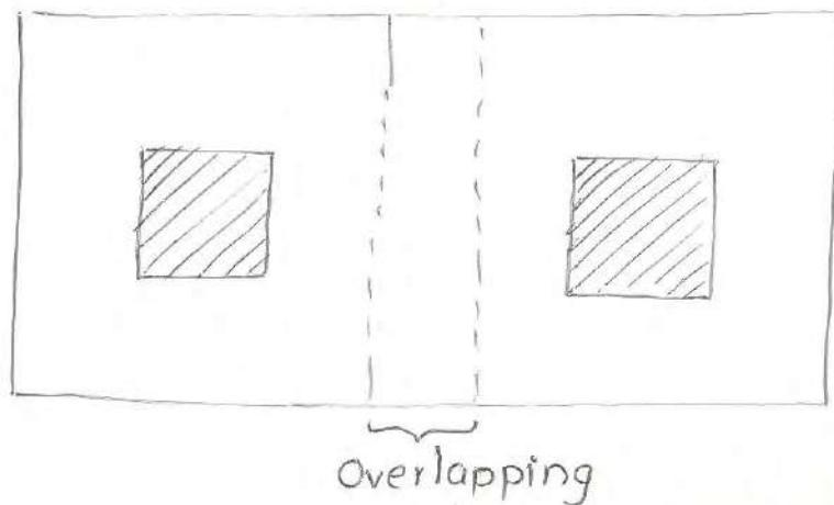
Case II: If column is placed at land boundary then its isolated footing is combined with isolated footing of other column to get desired pressure distribution for economical design.
