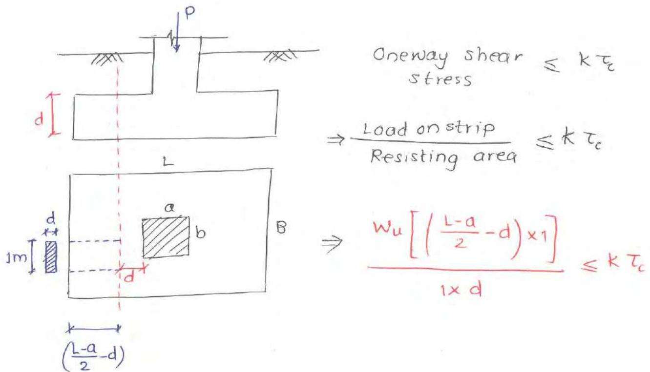
Above expression is used to calculate ' $d$ ' required to prevent oneway shear failure.
