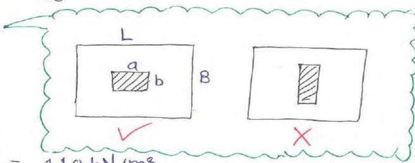
$$\text{Step 7: } w_{\text{net}} = \frac{P}{A_{\text{provided}}} = \frac{1200}{3 \times 4} = 100 \text{ kN/m}^2$$
