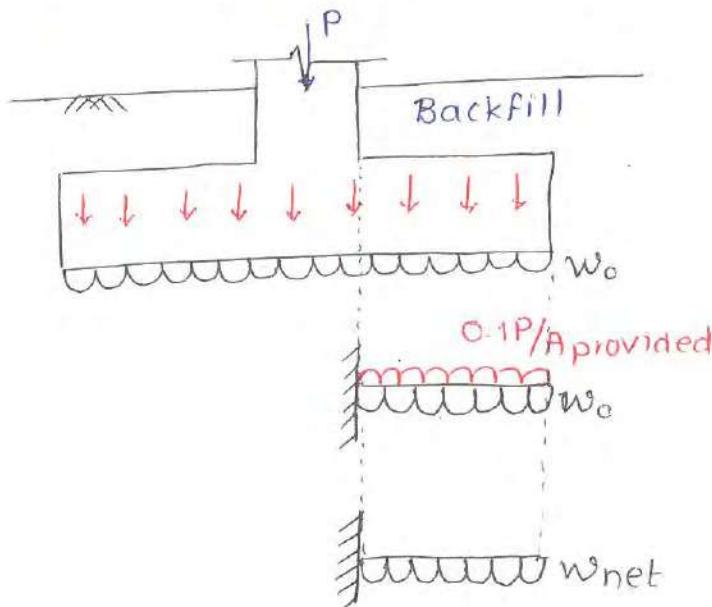
$$\begin{aligned} w_{net} &= w_o - \frac{0.1P}{A_{provided}} \\ &= \frac{P + 0.1P}{A_{prov.}} - \frac{0.1P}{A_{prov.}} \end{aligned}$$
