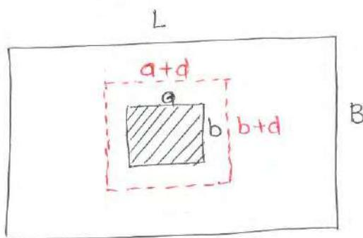
$\Rightarrow \frac{\text{Punching SF}}{\text{Resisting area}} \leq k_B 0.25 \sqrt{f_{ck}}$
