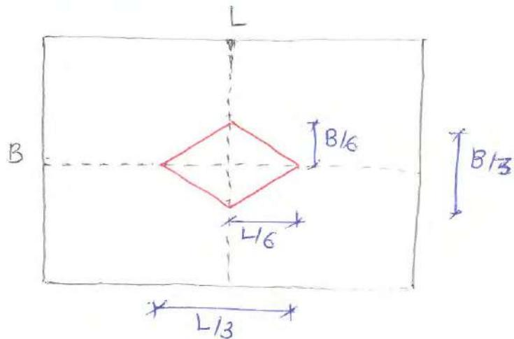
Ex. Calculate maximum and minimum pressure exerted by soil on footing base of plan area  $(3 \times 4)$  m. This footing is supporting axial load 2000 kN and moment 400 kNm about shorter side, at its base.
