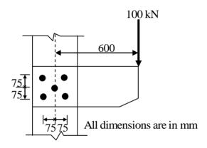
The maximum force for which the bolts should be designed is \_\_\_\_\_ kN.
