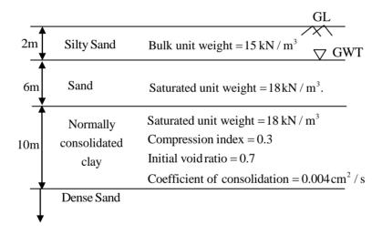
A circular footing of diameter 3m and depth of embedment 1m has been designed to support the tank. The total vertical load to be taken by the footing is 1500 kN. Assume the unit weight of water as  $10 \text{kN}/\text{m}^3$  and the load dispersion pattern as 2 V:1 H. The expected settlement of the tank due to primary consolidation of the clay layer is \_\_\_\_ mm.
