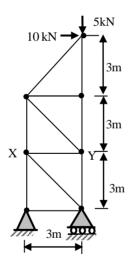
For member XY, assume AE = 30 kN, where A is cross-section area and E is the modulus of elasticity.
