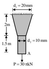
Both bars are made of same material with the modulus of elasticity,  $E = 2 \times 10^5$  MPa. When subjected to a load  $P = 30\pi$  kN, the deflection at point A is \_\_\_\_\_ mm.
