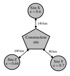
Assume the specific gravity of soil to be 2.7 for all three sites. If the cost of transportation per km is twice the cost of excavation per  $m^3$  of borrow pits, which site would you choose as the most economic solution? (Use unit weight of water =10 kN/m<sup>3</sup>).
