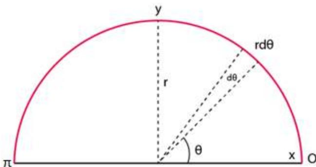
The force on particle due to element =  $dF = GmdM/r^2 = (GMm\pi d\theta)/L^2$
