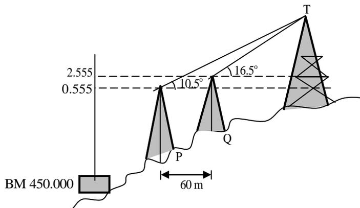
The two stations are in line with the tower and spaced at a distance of 60m. Readings taken from these two stations on a leveling staff placed at the benchmark (BM = 450.000 m) are also shown in the figure. The reduced level of the top of the tower T (expressed in m) is \_\_\_\_\_.
