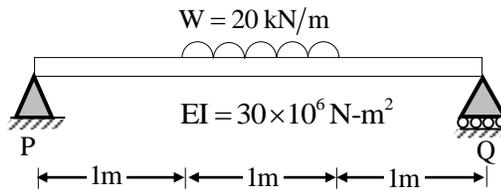
If the flexural rigidity ( $EI$ ) of the beam is  $30 \times 10^6 \text{ N-m}^2$ , the maximum slope (expressed in radians) of the deformed beam is
