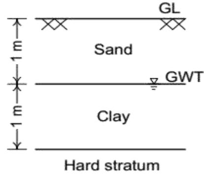
A compacted fill of 2.5 m height with unit weight of  $20\text{kN/m}^3$  is placed at the ground level.
