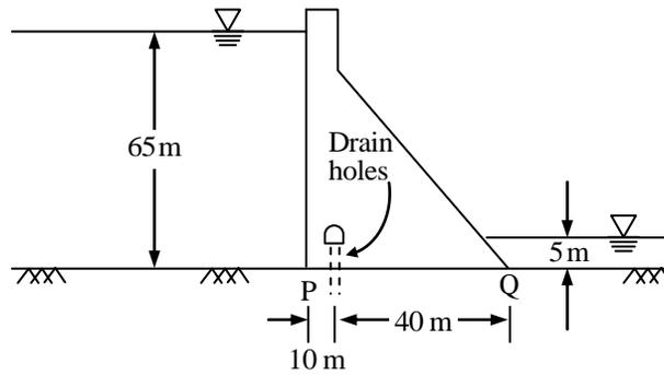
Assuming unit weight of water as  $10\text{kN/m}^3$  and unit weight of concrete as  $24\text{kN/m}^3$ , the uplift force per unit length of the dam (expressed in  $\text{kN/m}$ ) at PQ is \_\_\_\_\_.
