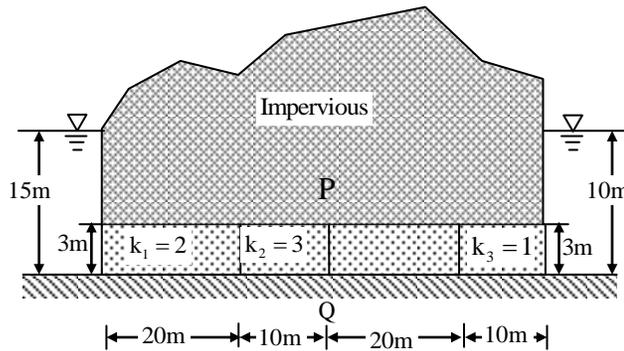
The seepage discharge ( $\text{m}^3/\text{day}$  per m) through the porous media at section PQ is
