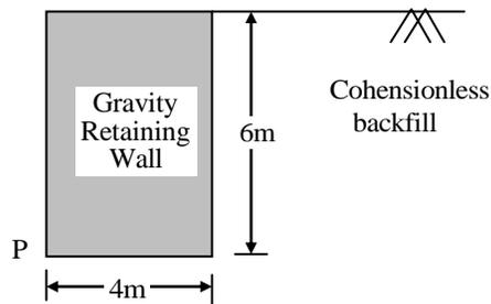
The minimum weight of the wall (expressed in kN per m length) required to prevent it from overturning about its toe (Point P) is
