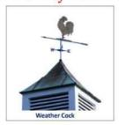
The device weathercock is used to show the direction in which air is moving at that place. In this device a cock is fixed on an arrow which is attached to a rotating axis. When air pushes the cock, the cock and its arrow rotate and align in the direction of moving air.
