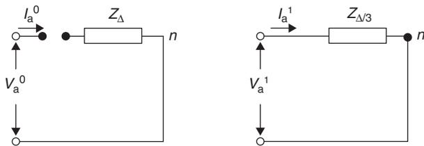
Figure 8 Positive sequence circuit
