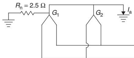
The positive, negative and zero sequence reactances are, respectively,  $j0.20$ ,  $j0.16$ ,  $j0.12$  p.u. The star point of one of the generator is isolated and that of the other is earthed through a  $2.5 \Omega$  resistor. A single line to ground fault occurs at the terminals of one of the generators
