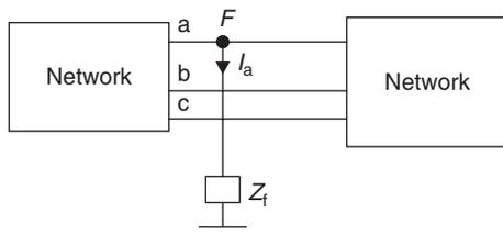
At the point of fault occurrence, the currents come out of the network and line to ground voltages are given by
