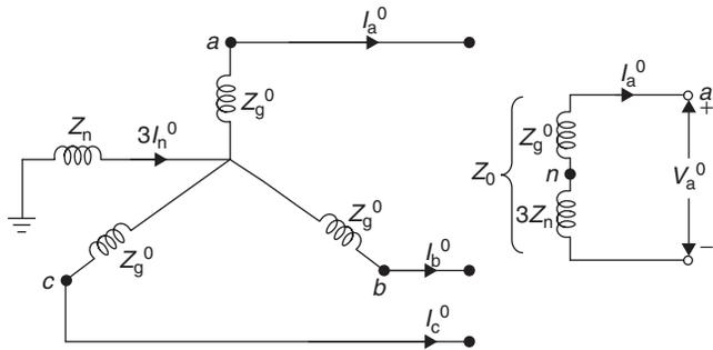
Figure 3 Zero-sequence network and its single-phase equivalent
