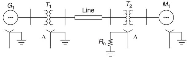
Which one of the following is the zero-sequence equivalent of the above system?
