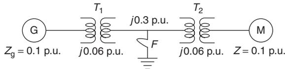
The system is on no load when three-phase fault occurs at  $F$  on the high voltage side of the transformer  $T_2$ . The fault current will be
