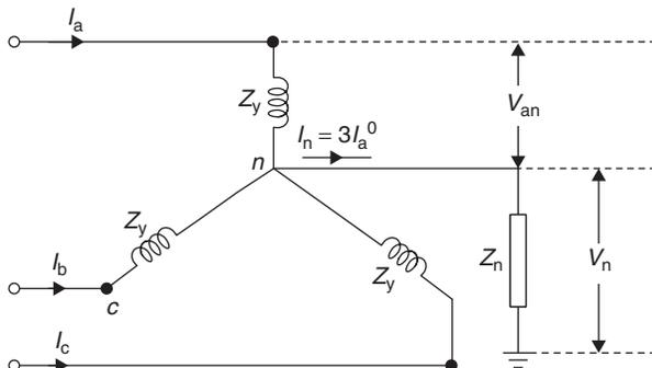
In the above Y-connected load, sum of the line current is equal to the neutral current  $I_n$  and it is given by
