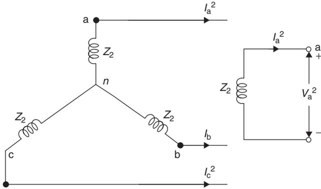
Figure 2 Negative-sequence network and its single-phase equivalent
