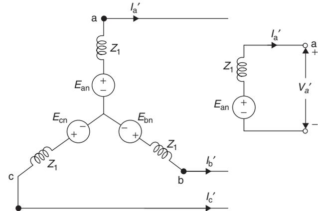
Figure 1 Positive-sequence network and its single-phase equivalent
