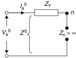
Figure 7 Zero sequence circuit
