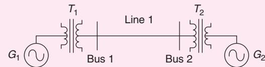
Choose 25 kV as the base voltage at the generator  $G_1$ , and 200 MVA as the MVA base. The impedance diagram is [2010]
