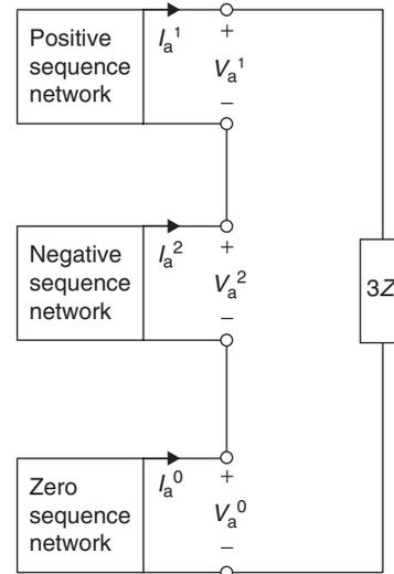
Figure 16 Sequence connection for LG Fault
