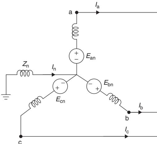
When the fault takes place at the terminals, the current  $I_a$ ,  $I_b$  and  $I_c$  flows in the lines. Whenever the fault involves ground, the total current  $I_a + I_b + I_c = I_n$  flows into the neutral of the generator and the line currents can be resolved into symmetrical components.
