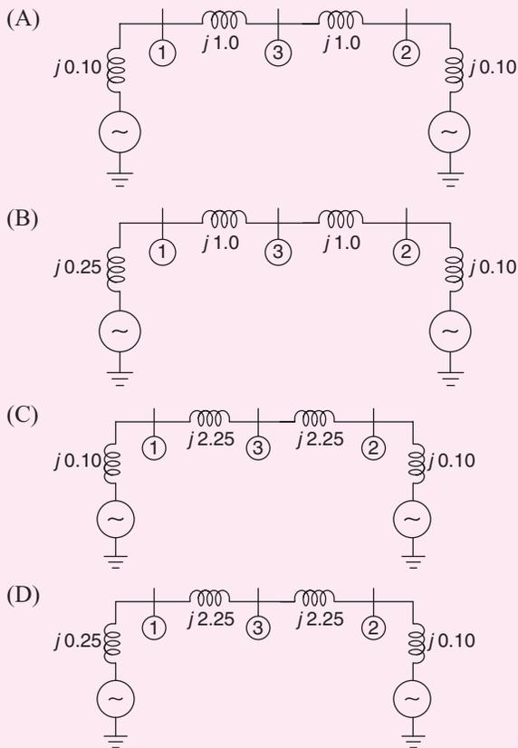
20. In the above system, the three-phase fault MVA at the bus 3 is [2011]
