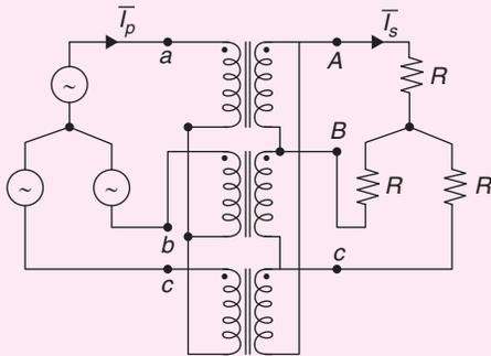
line voltage rating is 230 V on the star side, and 115 V on the delta side. If the magnetizing current is neglected and  $I_s = 100 \angle 0^\circ$  A, then what is the value of  $I_p$  in Ampere? [2015]
