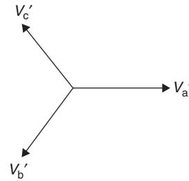
2. Negative-sequence components consisting of three phasors equal in magnitude, displaced from each other by  $120^\circ$  in phase, and having the phase sequence opposite to that of the original phasors.
