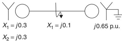
Prior to fault, the network is balanced and voltage at fault location is  $1\angle 0^\circ$  p.u. The current through the fault path is
