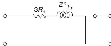
**Example 10:** A generator is connected to a transformer which feeds another transformer through a short transmission line. The zero-sequence impedances values are expressed in p.u. on a common base and are indicated in
