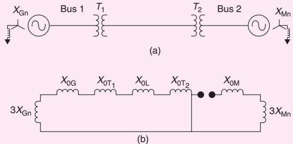
The transformers  $T_1$  and  $T_2$  are connected as [2014]
