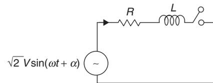
The above figure shows the RL circuit supplied by a voltage source according to given assumptions.
