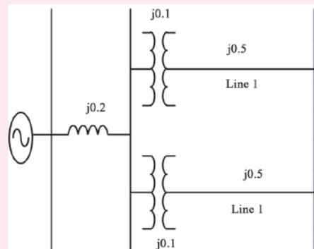
32. Two identical unloaded generators are connected in parallel as shown in the figure. Both the generators are having positive, negative and zero sequence impedances of  $j0.4$ pu.,  $j0.3$ pu., and  $j0.15$ pu., respectively. If the pre- fault voltage is 1pu, for a line - to - ground (L - G) fault at the terminals of the generators, the fault current, in pu., is \_\_\_\_\_.
