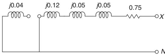
Equivalent impedance at point 'X' is,  $Z_{X_n} = j0.22 + 0.75$
