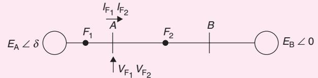
If the fault takes place at location  $F_1$ , then the voltage and the current at bus A are  $V_{F_1}$  and  $I_{F_1}$ , respectively. If the fault takes place at location  $F_2$ , then the voltage and the current at bus A are  $V_{F_2}$  and  $I_{F_2}$ , respectively. The correct statement about voltages and currents during faults at  $F_1$  and  $F_2$  is
