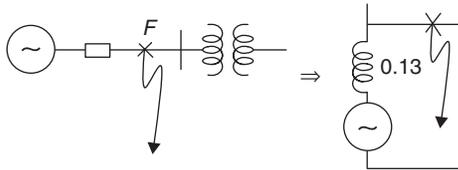
$$\text{Fault current } I_f = \frac{E}{X_d''} = \frac{1}{0.13} = 7.69 \text{ p.u.}$$
