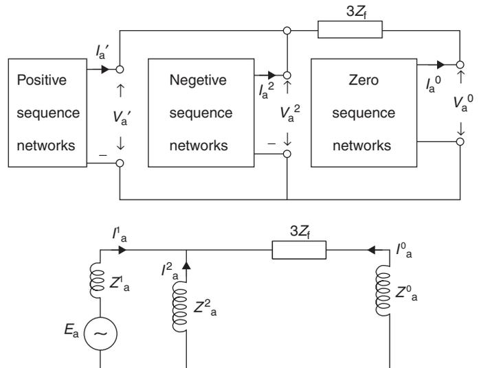
**Figure 18** Sequence-network connections and their Thevenin's equivalent network
