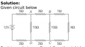
Resistance between  $B \mbox{ and } C$  on the right hand side of the circuit
