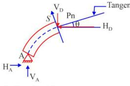
$V_D \rightarrow$  net vertical reaction at D  $H_D \rightarrow$  net horizontal reaction at D  $\theta \rightarrow$  angle b/w the tangent at D and horizontal
