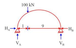
Horizontal reaction is not influencing the vertical reaction as their line of action through the support
