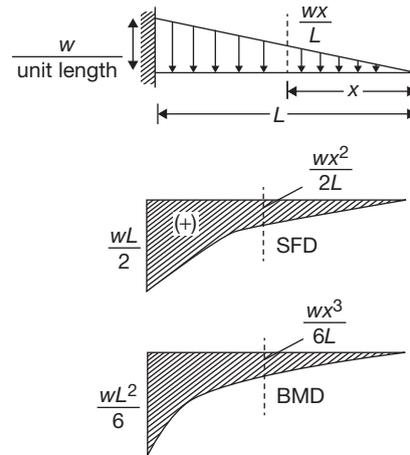
Shear force has a parabolic variation and bending moment has a cubic variation.
