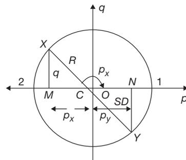
Draw line  $XY$  and locate the mid-point  $C$  the centre of Mohr's circle with  $C$  as the centre and radius equal to  $CX$  or  $CY$ , draw a circle which is the Mohr's circle.
