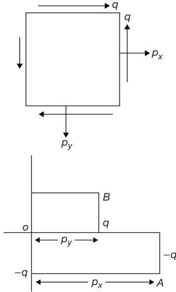
Mohr's circle is drawn on a set of axes representing normal stress (x-direction) and shear stress (y-direction).
