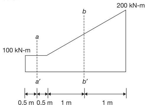
The shear force at sections  $aa'$  and  $bb'$  respectively are of the magnitude
