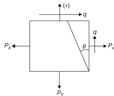
The plane makes angle  $\theta$  in the anti-clockwise direction from plane at which  $p_x$  acts. As per the sign convention, radial vector will be above the  $X$ -axis in positive direction.
