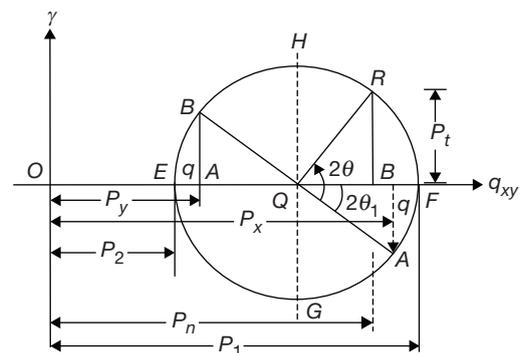
Line  $AB$  is a reference line representing  $p_x, p_y$  and  $q$ . Line  $QR$  is drawn at an angle twice  $\theta$  (i.e.,  $2\theta$ ). Coordinates of  $R$  give the values of normal stress  $p_x$  and shear stress  $p_t$  on the plane.
