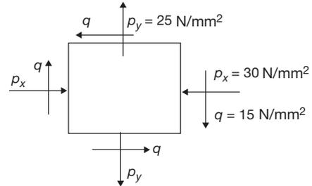
To draw the Mohr's circle, first draw a horizontal line representing the normal stress and then a vertical line representing the shearing stress. The point of intersection of these lines is the origin  $O$ , the point from where the stress values are plotted.
