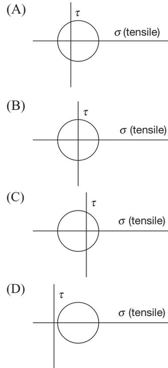
9. The state of two dimensional stresses acting on a concrete lamina consists of a direct tensile stress,  $\sigma_x = 1.5 \text{ N/mm}^2$ , and shear stress,  $\tau = 1.20 \text{ N/mm}^2$ , which cause cracking of concrete. Then the tensile strength of the concrete in  $\text{N/mm}^2$  is
