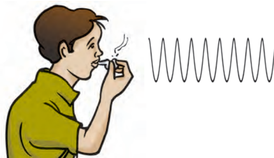
Fig. 13.18 : Frequency determines the pitch of a sound
