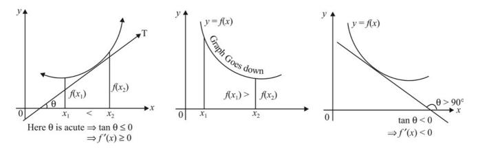
if f(x) be real valued continuous function defined on (a, b) is said to be decreasing in (a, b) if  $x_1, x_2 \in (a, b)$  such that  $x_1 < x_2 \Rightarrow f(x_1) > f(x_2)$
