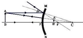
Use of convex mirror—as rear view mirror in vehicles Why—always gives erect image with large field of view
