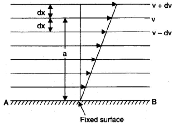
**Fig. 12.01.** Relative motion between different layers.
