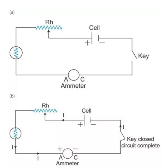
(c) A rheostat is used to control the current in the circuit.
