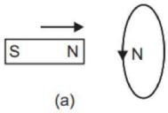
Similarly when north pole of the magnet is moved away from the coil, the direction of current in the coil will be such as to attract the magnet. For this the nearer face of coil behaves as south pole. This necessitates a clockwise current in the coil, when seen from the magnet side (fig. b).
