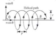
The plane of the circle is perpendicular to the magnetic field and the axis of the helix is parallel to the magnetic field. The charged particle moves along helical path touching the line parallel to the magnetic field passing through the starting point after each rotation.
