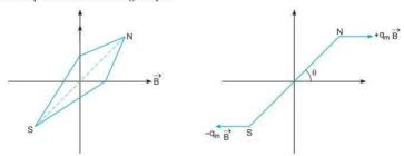
Restoring torque,  $\vec{\tau} = -$  magnetic force  $\times$  perpendicular distance  $= -q_m B \cdot (2a \sin \theta)$ ,
