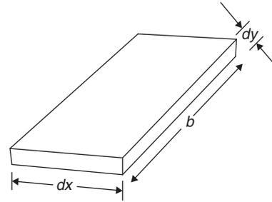
In a beam, consider an elemental length of length  $dx$ . Moments acting at the two sides of this element =  $M$  and  $M + dM$
