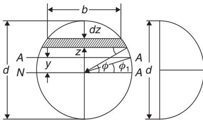
In the given circular section of diameter  $d$ , shear stress is to be determined at a section  $AA$  at a distance  $y$  from the neutral axis  $NA$ .
