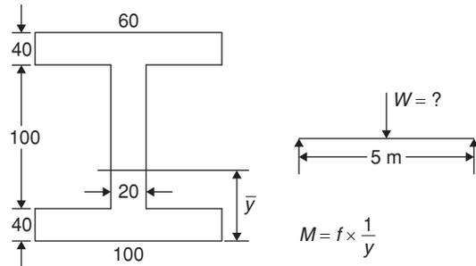
Moment carrying capacity of the beam is to be found out. For this distance  $y$  from centroid is to be found out for both tension and compression. So position of centroid is to be located first.
