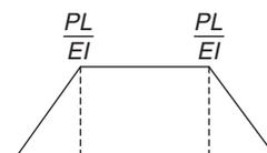
$$\begin{aligned} \text{Strain energy stored} &= \int \frac{M^2}{2EI} dx \\ &= 2 \int_0^L \frac{(Px)^2}{2EI} dx + \int_0^L \frac{(PL)^2}{2EI} dx \\ &= \frac{P^2}{2EI} \left[ \frac{2x^3}{3} + L^2 \cdot x \right]_0^L \\ &= \frac{P^2}{2EI} \left[ \frac{2}{3} L^3 + L^3 \right] \\ &= \frac{P^2}{2EI} \times \frac{5}{3} L^3 \\ &= \frac{5P^2 L^3}{6EI} \end{aligned}$$
