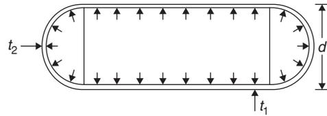
Consider a cylindrical pressure vessel with hemispherical ends of internal diameter  $d$  subjected to an internal pressure  $p$ . Let  $t_1$  be the thickness of cylindrical portions and  $t_2$  be the thickness of the hemispherical portion.
