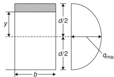
In the above expression,  $q$ , the shear stress is at a distance  $y$  from the neutral axis  $a\bar{y}$  is the moment of area above this section.
