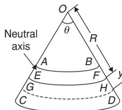
After bending, cross sections  $AC$  and  $BD$  subtends an angle  $\theta$  at  $O$ . Let  $R$  be the radius of the neutral plane represented by  $EF$ . Then  $EF = R\theta$
