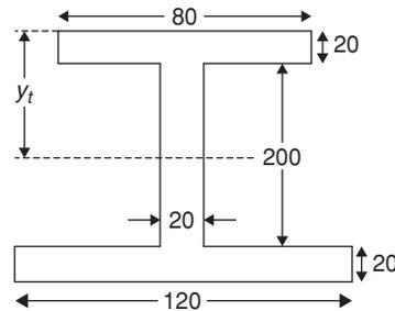
The shear stress at the bottom of the top flange will be
