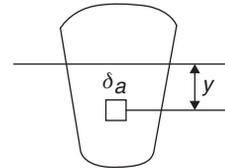
Considering an element of area  $\delta a$  at a distance  $y$  from the neutral axis,
