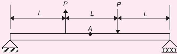
It is given that  $P = 1$  N,  $L = 1$  m and Young's modulus  $E = 200$  GPa. The cross-section is a square with dimension  $10 \text{ mm} \times 10 \text{ mm}$ . The bending stress (in Pa) at the point  $A$  located at the top surface of the beam at a distance of  $1.5L$  from the left end is \_\_\_\_\_.
