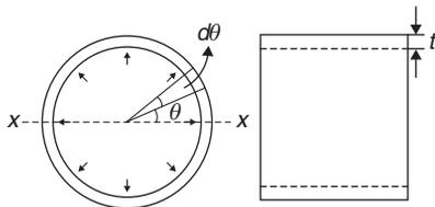
Due to the internal fluid pressure on the wall of the cylinder the following types of stresses are developed:
