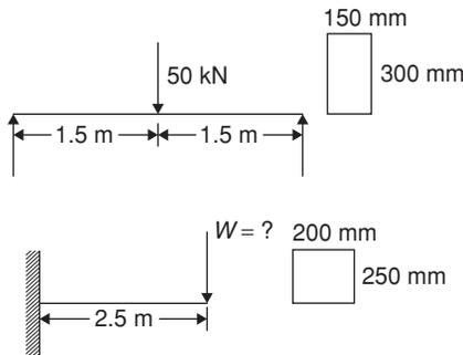
$$\begin{aligned} \text{Maximum moment in simply supported beam} &= \frac{WL}{4} \\ &= \frac{50 \times 3}{4} = 37.5 \text{ kNm} = 37.5 \times 10^6 \text{ Nmm} \end{aligned}$$
