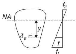
Stress is varying linearly across the depth. Consider an elemental area  $\delta a$  at a distance  $y$  from the neutral axis. Let  $f$  be the stress on this area.
