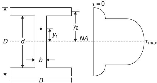
The I-section is symmetric about neutral axis and shear stress  $q$  is maximum at neutral axis (NA).
