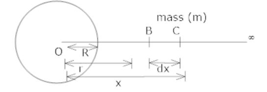
A body of mass (m) lying at a distance x from earth of mass (m)
