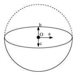
Since gravitational intensity at a point is defined as the gravitational force per unit mass at that point, it will also act in the downward direction. Thus, the gravitational intensity at centre O of the given hemispherical shell has the direction as indicated by arrow **c**.
