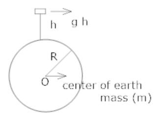
If g h is the acceleration due to gravity at a pt situated at a height 'h' above the surface of the earth
