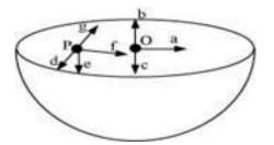
Ans. (iii)Gravitational potential (V) is constant at all points in a spherical shell. Hence, the gravitational potential gradient  $\left(\frac{dV}{dr}\right)$  is zero everywhere inside the spherical shell. The gravitational potential gradient is equal to the negative of gravitational intensity. Hence, intensity is also zero at all points inside the spherical shell. This indicates that gravitational forces acting at a point in a spherical shell are symmetric.
