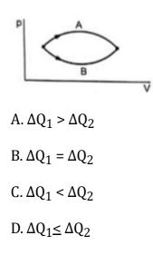
Initial and final points of both processes A and B are same. Therefore, internal energy in both the processes will be the same because internal energy is a state variable, independent of the path taken.
