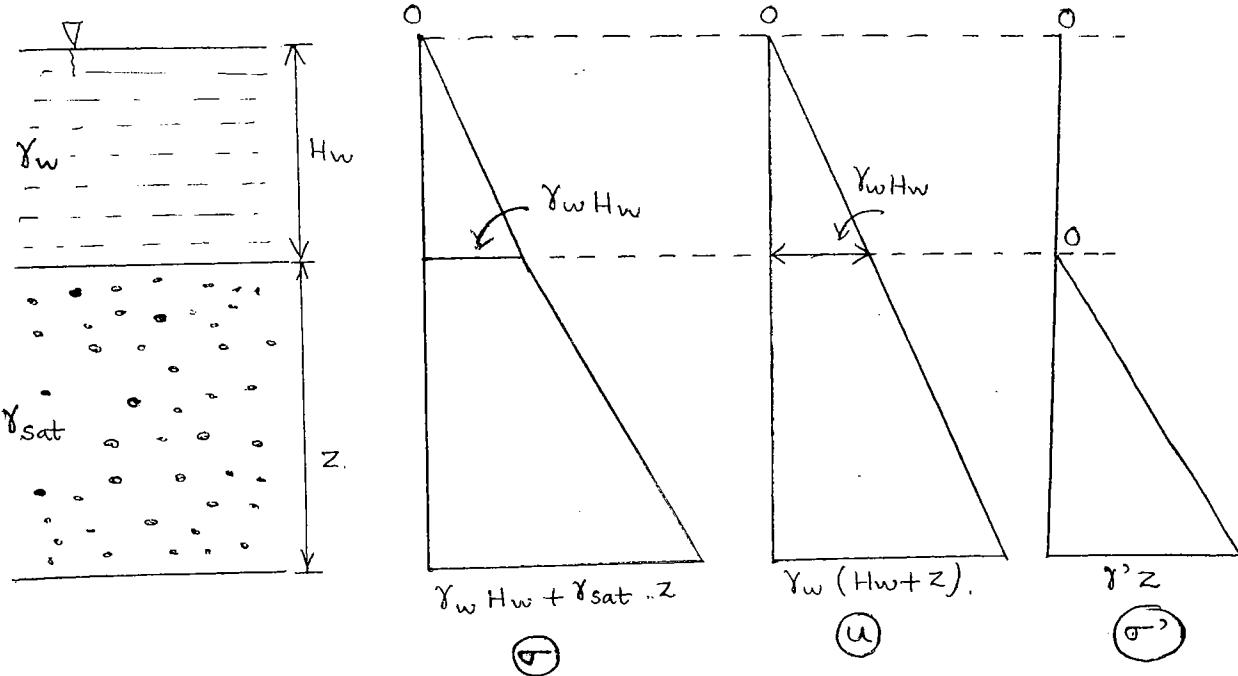
④ Effective stress below the bed level is totally independent of depth of water ( $H_w$ ) above bed level.
