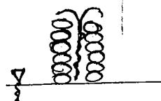
Soil molecules act like walls of the capillary tube and they are under compression.  $\therefore \sigma'$  increases in capillary zone.
