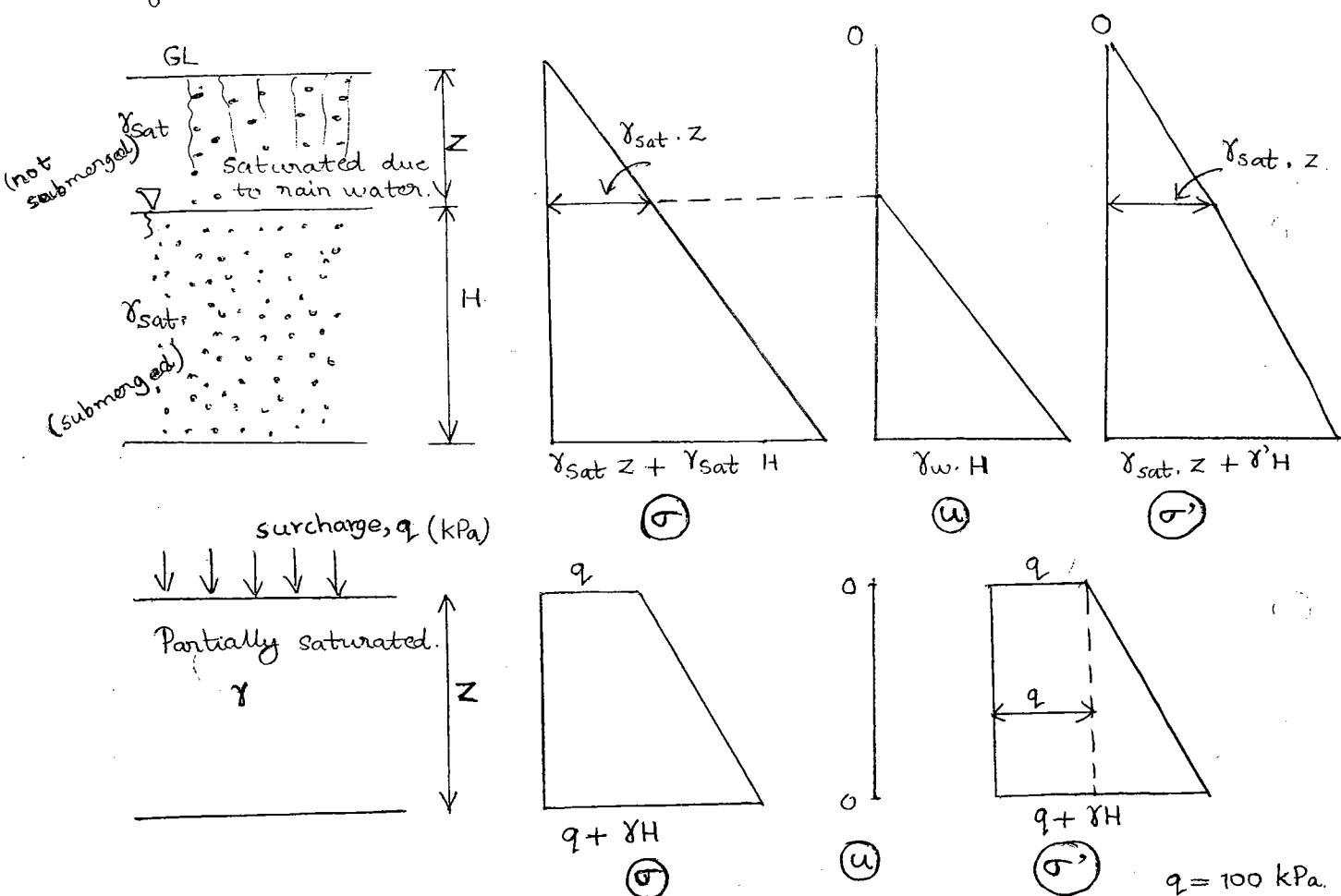
Above stress distribution diagrams are possible only if surcharge is infinite
