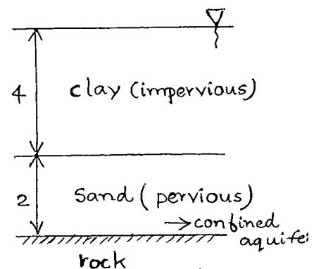
Springs are developed only when piezometric surface is above GL.
