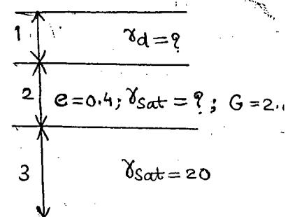
Q. 7 b) Calculate  $\sigma'$  at a depth of 2.4 m below GL for the above capillarity case.
