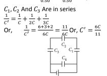
As the capacitors  $\mathcal{C}_{\rm 1},\mathcal{C}_{\rm 2}$  And  $\mathcal{C}_{\rm 3}$  Are in series so the charge on each capacitor is
