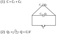
$$Q_2 = \frac{C_2}{C_1 + C_2} Q = C_2 V$$
