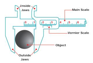
Figure 1.2 Vernier Caliper
