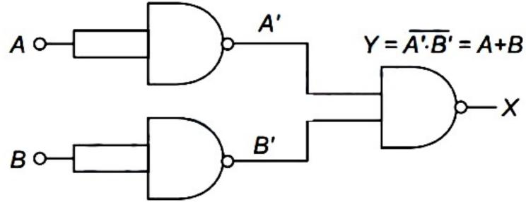
The following combination of gates is equivalent to OR gate.
