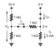
$$\begin{split} \frac{V_X - 10}{1 \text{k}\Omega} + \frac{V_X - 3}{1 \text{k}\Omega} + \frac{V_X}{1 \text{k}\Omega} &= 0 \\ 3V_X &= 13 \\ V_X &= \frac{13}{3} &= 4.33 \text{ V} \\ I_1 + I_{D1} &= I_2 \\ \frac{4.33 - 3}{1 \text{k}\Omega} + I_{D1} &= 3 \text{ mA} \\ I_{D1} &= 3 \text{ mA} - 1.33 \text{ mA} \\ &= 1.67 \text{ mA} \end{split}$$
