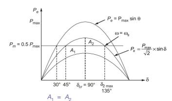
$$\int_{90^{\circ}}^{135^{\circ}} \left( \frac{P_{\text{max}}}{\sqrt{2}} \sin \delta - 0.5 P_{\text{max}} \right) d\delta = 0.1 P_{\text{max}}$$
