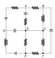
A point at which more than two elements are joints together is called Junction. A, B, C, D, E and F are junction.
