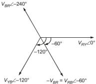
$$V_{RY} = 400 \angle 0^{\circ}$$
