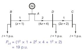
By opening branch  $b_3$  Power loss is minimum.
