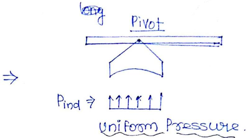
★  $\Rightarrow$  long shoe is pivoted on the lever to minimise wear.
