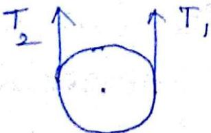
$$T_f = (T_1 - T_2) \times R \quad \text{--- (1)}$$
