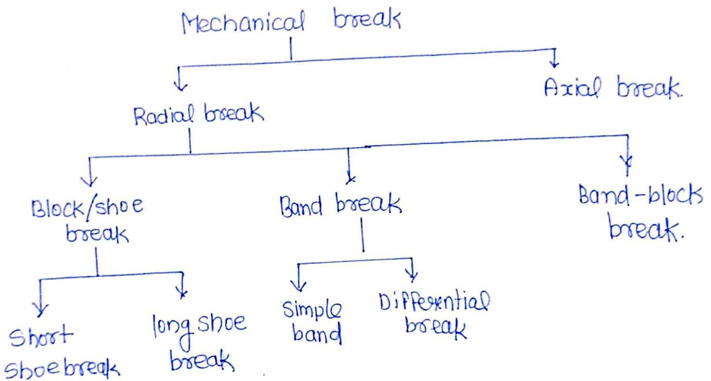
Radial break  $\Rightarrow$  force applied for breaking in Radial dir<sup>n</sup>.
