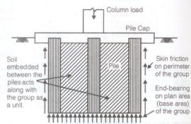
Single equivalent large pile concept for a group (block failure)
