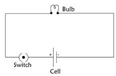
A diagram which shows how different components in a circuit have been connected using conventional symbols for the components is called a circuit diagram.
