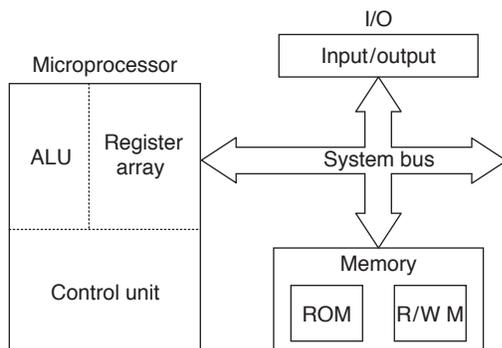
Microprocessor-based systems include three components: microprocessor, input/output (I/O) and memory
