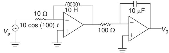
In the figure, assume the OP-Amps to be ideal. The output  $V_0$  of the circuit (in mV) is
