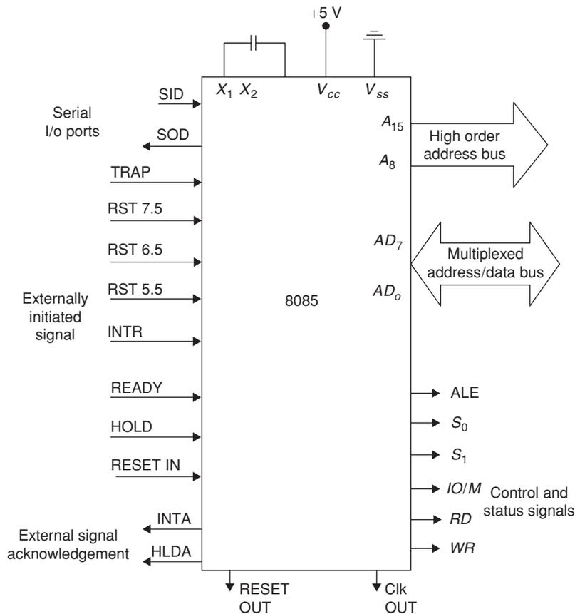
Figure 3 The 8085 microprocessor signals
