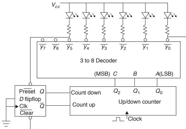
Assume that initial values of counter output ( $Q_2Q_1Q_0$ ) as zeros. The counter output in decimal for next 12 clock cycles are
