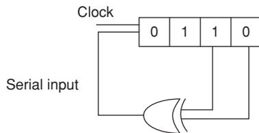
Initial contents of the 4-bit serial-in-parallel out right shift, shift register as shown in figure are 0110. After three clock pulses, the contents of the shift register will be
