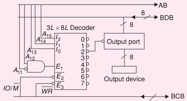
The interfacing circuit makes use of 3 line to 8 line decoder having 3 enable lines  $E_1, \bar{E}_2, \bar{E}_3$ . The address of the device is
