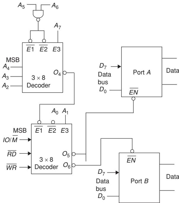
**Solutions:** Two ports port A, and port B are connected in the above figure with two decoders.
