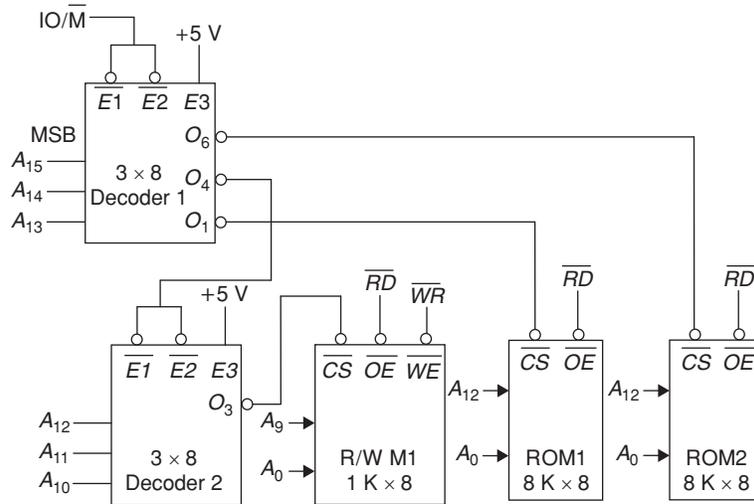
**Solution:** ROM1, ROM2 are read only memories  $\overline{OE}$  —output enable is connected to  $\overline{RD}$  signal of microprocessor. The chip select of ROM1, ROM2 are given from  $3 \times 8$  decoder 1 outputs  $O_2$  and  $O_6$ .
