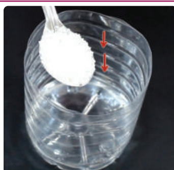
Fig. 2.8 , 50 ml of sugar solution is prepared with 7% concentration, i.e. 3.5 g sugar dissolved in 50 ml water
