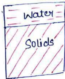
fully saturated Soil [2-phase Diagram]
