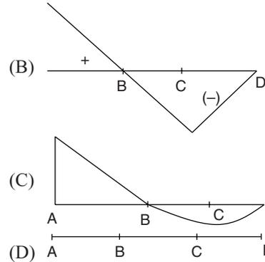
14. A beam *ABCD* is 15m long and is simply supported at *B* and *C* 8 m apart. Overhangs *BA* and *CD* are 3m and 4m respectively. A train of two point loads of 150 kN and 100 kN, 3 m apart, crosses the beam from left to right with 100 kN load leading. The maximum sagging *B.M.* under 150 kN load anywhere is
