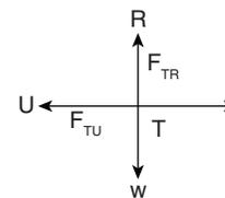
Three forces are acting at a joint; [i.e., W;  $F_{TR}$ ;  $F_{TU}$ ] and two of the forces are in same line i.e., W and  $F_{TR}$  the force in  $F_{TU}$  to be zero since for equilibrium of a joint
