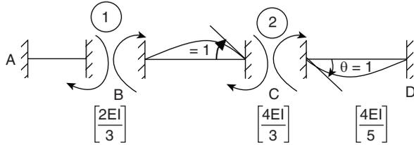
$$K_{22} = K_{22} = \left[ \frac{4EI}{L} \right]_{CB} + \left[ \frac{4EI}{L} \right]_{CD} = \left[ \frac{4E(2I)}{3} \right] + \left[ \frac{4EI}{5} \right]$$
