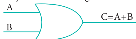
Fig. 2.5 Logic symbol of OR Gate
