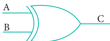
Fig. 2.16 Logic Symbol of XOR Gate
