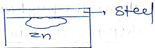
when a thin layer of Zn is coated over steel and if there is a small hole on surface concentration of  $e^-$  will be very high through this hole, this leads to rapid corrosion of anodic material.
