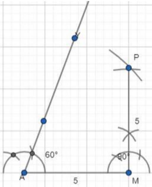
Step 4 : with center 'P' and radius 5cm ( $PL = 5$  cm) draw an arc to intersect PY at L. Join L,P . LAMP is the required quadrilateral.
