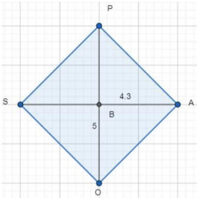
Step 2 : draw SA = 4.3cm (one diagonal of the rhombus SOAP) and draw a perpendicular bisector XY of it and mark the point of intersection as 'B'.
