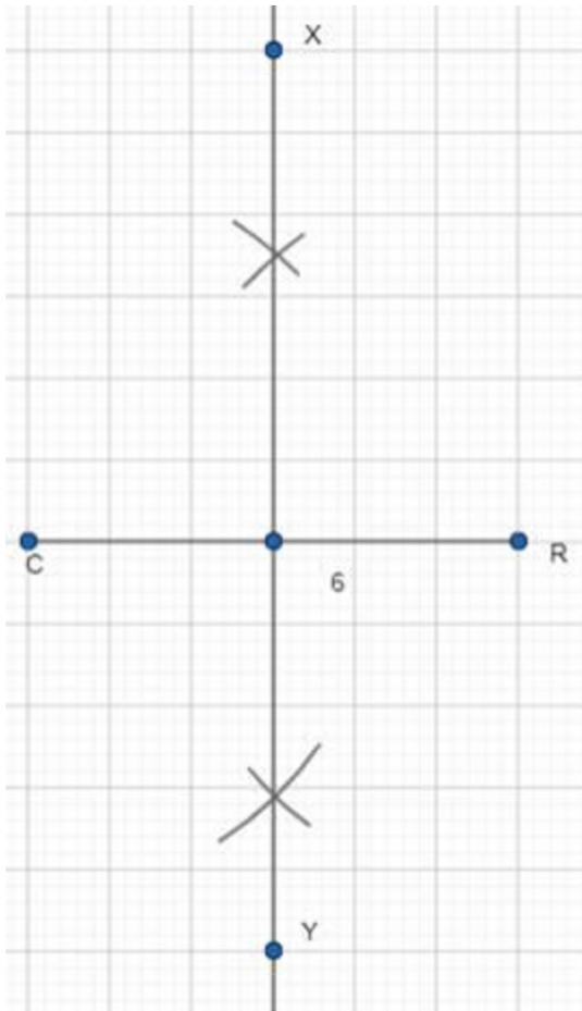
Step 3 : as the other diagonal AT is perpendicular to CR , AT is a part of XY. So, with center 'O' and radius 2.4 cm ( $AO = OT = 2.4\text{cm}$ ) draw 2 arcs on either sides of CR to cut XY at A and T.
