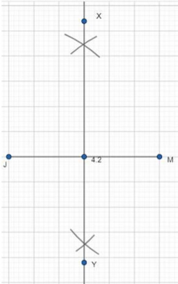
Step 3 : as the other diagonal UP is perpendicular to JM , UP is a part of XY. So, with center 'B' and radius 2.1 cm ( $OU = BP = 2.1\text{cm}$ ) draw 2 arcs on either sides of JM to cut XY at U and P.
