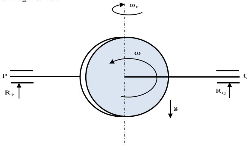
The disc spins counter-clockwise about the axle with angular speed  $\omega$ , when viewed from the right-hand side bearing Q, a The axle processes about a vertical axis at  $\omega_p = \omega/10$  in the clockwise direction when viewed from above. Let  $R_p$  and  $R_q$  (positive upwards) be the resultant reaction forces due to the mass
