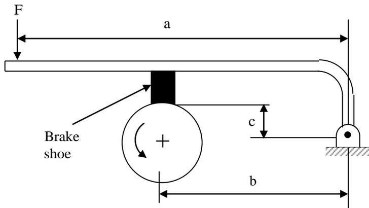
The force applied on the lever  $F = 100$  N as shown in the figure. The drum is rotating anti-clockwise. The braking torque on the drum is \_\_\_\_\_ N-m (roundoff to two decimal places).
