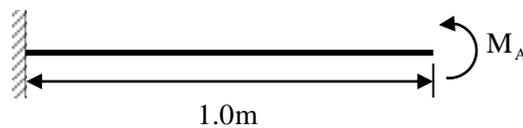
The magnitude of the vertical deflection of the free end is \_\_\_\_ mm (round off to one decimal place)
