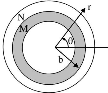
Similarly  $(u_r^N, u_\theta^N)$  and  $(\sigma_r^N, \sigma_{\theta\theta}^N)$  denote the radial and tangential displacement and stress components, respectively, in material N. The boundary condition that need to be satisfied at the frictionless interface between the two cylinders are:
