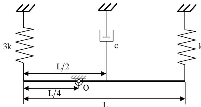
For the system to be critically damped, the ratio  $c / \sqrt{km}$  should be
