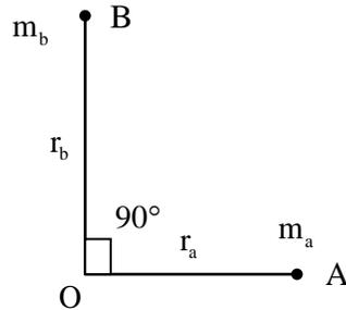
The radii of rotation of the masses  $m_a$  and  $m_b$  are  $r_a$  and  $r_b$ , respectively. The angle between lines OA and OB is  $90^\circ$ . If  $m_a = 10$  kg,  $m_b = 20$  kg  $r_a = 200$  mm and  $r_b = 400$ mm, then the balance mass to be placed at a radius of 200 mm is \_\_\_\_ kg (round off to two decimal places)
