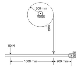
A band brake is used to control the speed of a flywheel as shown in figure. The coefficient of friction between the band and flywheel is 0.3. Radius of the flywheel is 300 mm. A force of 50 N is applied at the end of the lever as shown in the figure.
