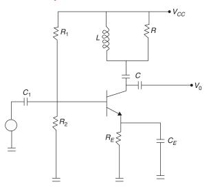
Class C amplifier is used to generate a pulse wave form whose conduction angle is less than 180°. Efficiency of class C amplifier is 90%.
