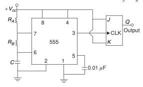
Figure 11 Symmetrical wave form generator.
