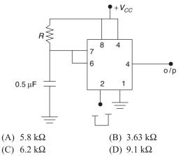
**41.** An astable multivibrator using *IC* 555 timer is given below; generate a square pulse of frequency 1 kHz with duty cycle 60%, what is the Relation between  $R_A$  and  $R_B$ ?
