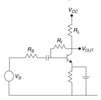
**Example 9:** The type of feedback used in this circuit is(A) Voltage shunt.(B) Current shunt.(C) Voltage series.(D) Current series.
