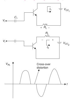
For positive values of sinusoidal input  $(V_1) Q_1$  conducts and  $Q_2$  is OFF  $(i_2 = 0)$  so that  $i_1$  is the positive half sine wave.
