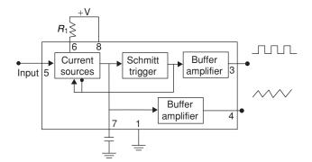
Figure 12 Block diagram. of 566
