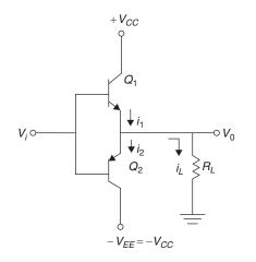
Figure 9 A complementary common-emitter push-pull amplifier
