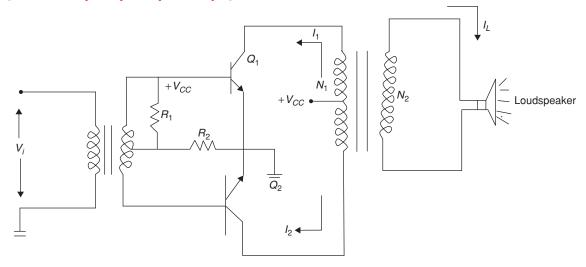
During positive half cycle:  $Q_1$  ON and  $Q_2$  OFF Negative half cycle:  $Q_1$  OFF and  $Q_2$  ON
