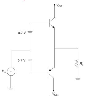
Cross over distortion is eliminated by adding two diodes whose cut in voltages were +0.7 V and -0.7 V.
