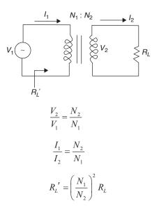
**Example 5:** Calculate the effective resistance seen looking into the primary of a 15:1 transformer connected to an 8  $\Omega$  load
