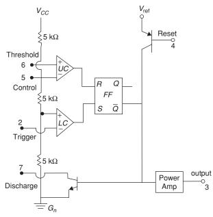
Figure 10 Functional diagram of 555 timer
