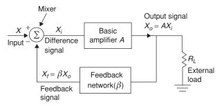
Figure 5 Schematic representation of a single loop feedback amplifier
