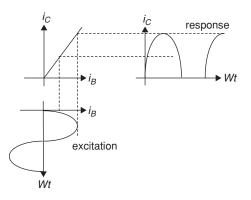
Figure 6 Emitter follower with zero bias operating as class B amplifier
