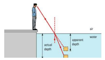
2. A straight stick which is immersed partly in water always looks to be bent at the surface of the water, because the light coming from the stick bends when it comes out at the surface due to refraction of light. The figure below illustrates it.
