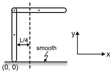
centre of mass does not move in x-direction as  $\Sigma F_x = 0$ .
