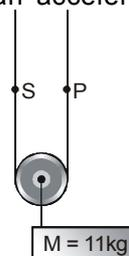
The point P has an acceleration  $a$  upwards, the block has an acceleration  $a$  downwards so the acceleration of S will be  $3a$  downwards. (because
