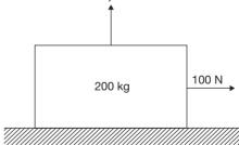
A body of mass 200 kg rests on a horizontal surface as shown in the figure. Coefficient of friction between the body and surface is 0.2. If a horizontal pull of 100 N can be exerted on the body, the vertical force P required to move the body is
