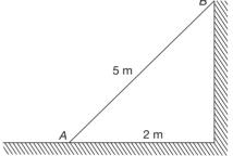
A uniform ladder of length 5 m and weight 250 N is placed against a smooth vertical wall with its lower end 2 m from the 00wall. Coefficient of friction between floor and ladder is 0.25. Friction at the wall may be neglected. Frictional force at A, the bottom of ladder is
