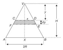
Consider one such disc of radius x, thickness dy and at a depth y from the vertex of the cone, i.e., from V.
