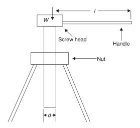
It mainly consists of a nut which forms the body of the jack and a screw is fitted into it. The threads are generally square. The load 'W' is placed on the head of the screw. By rotating the screw with a handle the load is lifted or lowered. Let W be the load lifted,  $\alpha$  be the angle of helix of the screw and  $\phi$ be the angle of friction.
