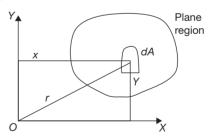
The moment of inertia of the area about the X-axis and Y-axis are
