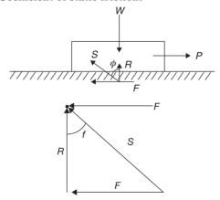
It is defined as the ratio of the limiting force of friction (F) to the normal reaction (R) between two bodies (see the above figure, where a solid body rests on a horizontal plane). It is denoted by  $\mu$ .
