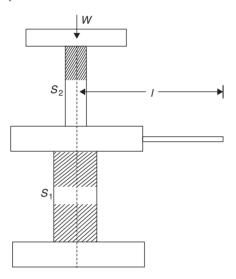
This spindle carries both internal as well as external threads. The spindle  $S_2$  is engaged to spindle  $S_1$  by means of an internal thread. When spindle  $S_1$  ascends, spindle  $S_2$  descends. This is also known as 'differential screw' jack. The principle of working of this jack is similar to the one as described in the given figure.
