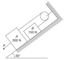
Two blocks A and B weighing 300 N and 150 N respectively are placed on a rough inclined plane of angle 30° and connected through a string over a pulley as shown in the figure. Coefficient of friction of the contact surfaces are 0.25. Force P required on block A for impending motion of the blocks is
