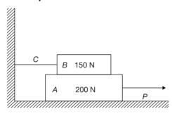
Block A weighing 200 N is placed on plane floor and block B weighing 150 N is placed over block A. Block B is constrained by a string C and a force P is applied on block Aas shown in figure. For the contact surfaces, coefficient of static friction is 0.3 and coefficient of kinetic friction is 0.25.
