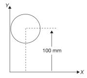
If the density of the material making up the circular crosssection is 7800 kg/m<sup>3</sup>, the weight of the ring generated is
