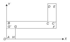
The X-axis and Y-axis of reference are chosen as shown in the above figure such that origin O coincides with point A of the figure and the axes coincide with the leftmost and bottommost lines of the figure, respectively. The position of the centre of gravity is determined with respect to origin O.
