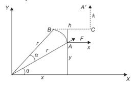
To illustrate the principle of work, let us consider a body at equilibrium at a point A. A force 'F' acts on the body and displaces it to the point A', where the displacement consisting:
