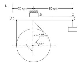
A rotating wheel is braked by a belt AB attached to the lever ABC hinged at B. The coefficient of friction between the belt and the wheel is 0.5. The braking moment exerted by the vertical weight W = 200 N is
