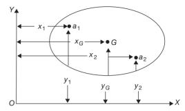
The above figure shows an irregular lamina of total area 'A' whose centre of gravity is to be determined. Let the lamina be composed of small areas  $a_1, a_2, ...,$  etc., such that:
