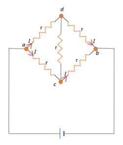
As we wish to find the resistance between points a and b, we have proceeded to add a voltage source of emf  $\epsilon$  between the points a and b.
