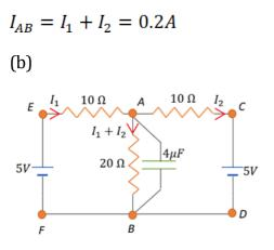
At steady state, no current passes through the capacitor; hence, the results are the same as in (a).
