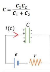
Let the potential across the capacitor C be at time t be  $V_{\rm c}.$  Let the charge at time t be q.
