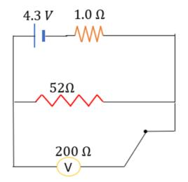
Note that the voltmeter and r' are in parallel.
