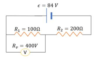
We can easily see that the voltmeter and  $R_1$  are in parallel. The equivalent resistance, r' is given by:
