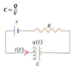
Let the potential across the capacitor be at time t be  $V_c$ . Let the charge at time t be q. The initial charge is Q.
