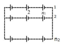
When  ${\rm n}_1$  cells each with emf 'E' are connected in series, the total emf,  ${\rm E}_{\rm net}$  in one branch is,
