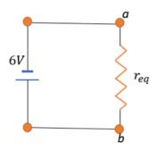
Where  $\boldsymbol{r}_{eq}$  has replaced the following infinite combination:
