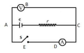
a) When switch is open, the current would circulate through loop ABCA but not through the loop ACDEA. Since the internal resistance is very small compared to the resistance of Voltmeter, the voltage drop occurs completely across the voltmeter. This voltage drop will be measured in the meter and it will be almost equal to the emf of the cell.
