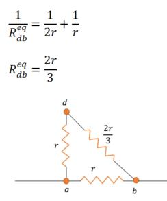
The resistor across *db* and *ad* are in series.
