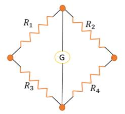
The condition for no deflection through the galvanometer is
