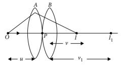
An object is placed at point *O*. The lens *A* produces an image at  $I_1$  which serves as a virtual object for lens *B* which produces final image at *I*.
