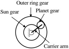
The ratio of magnitudes of angular velocity of the planet gear to the angular velocity of the carrier arm is
