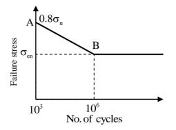
If the element is to be designed for a finite of 10000 cycles, the maximum amplitude of a completely reversed operating stress is  $\_\_\__N/mm^2$ .
