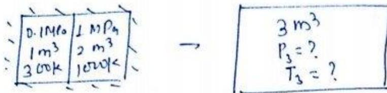
$$P_3 = \frac{P_1 V_1 + P_2 V_2}{V_1 + V_2} = \frac{0.1 \times 1 + 1 \times 2}{3}$$
